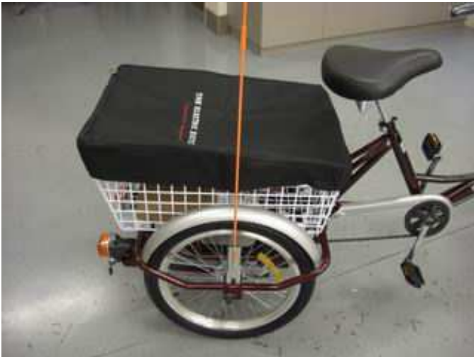
Using the four 5mm bolts attach the rear baskets to the trike.
