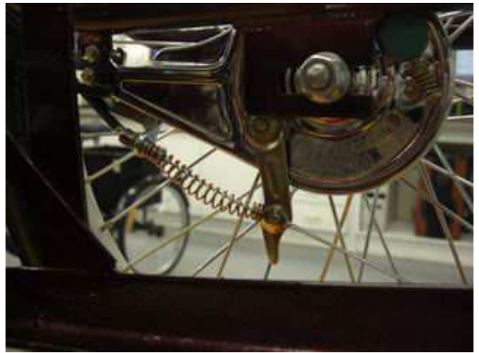
Poke the cable through the brass Brake adjuster. Ensure that you fit the spring between the adjuster and brake arm before locking up with appropriate tension using the 10mm nut. Be sure to secure both cables safely out of the way.
