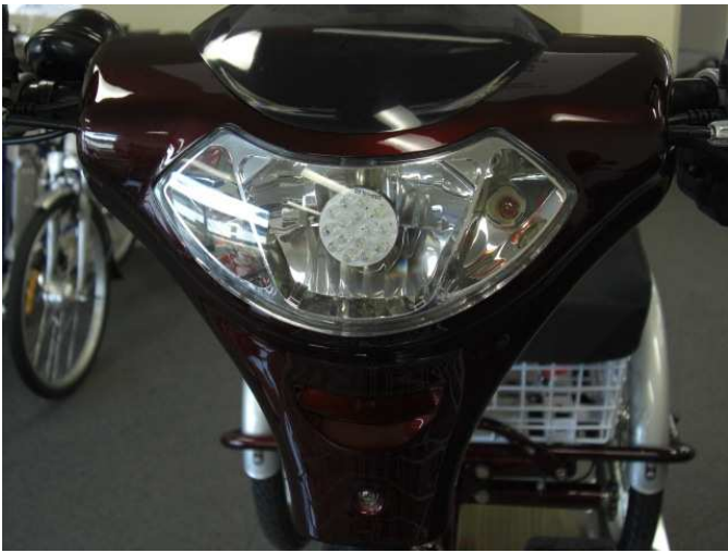
Refit the headpiece ensuring no wires get pinched.
