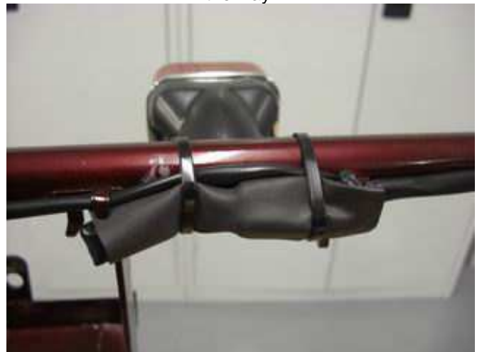
Once in place connect the plugs and secure excess wiring in a safe location under the frame using zip ties.
