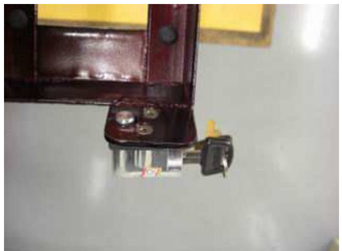
Attach rear battery lock.
