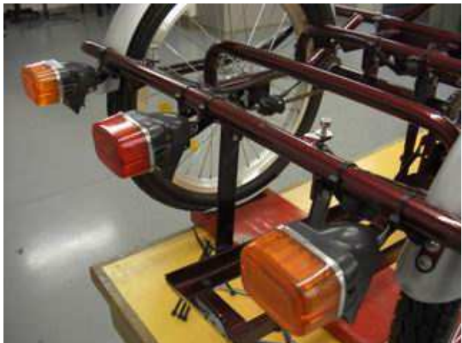
Now is a good time to fit the rear indicators and taillight. Attach using an 8mm ring-spanner.
